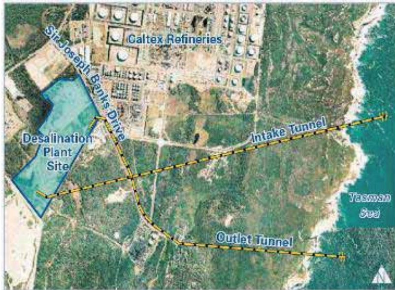
Location of seawater intakes and outlets
